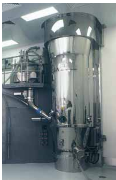
The outside of a fluid bed dryer.
