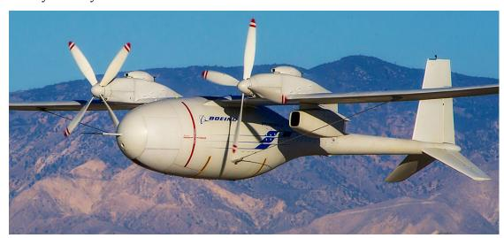
**Phantom Eyes – Communication High Altitude Platform (CHAP)** can instantly blanket a country with communications capabilities. Two in the sky continually can provide Papua New Guinea with a communications network. Fourteen such craft would blanket Africa with a further three spare on the ground.
